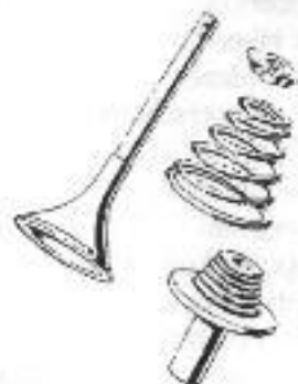
Tulip valves, finned guides, and conical springs were used on the early TT machines and the first production Big Ports of 1923.
